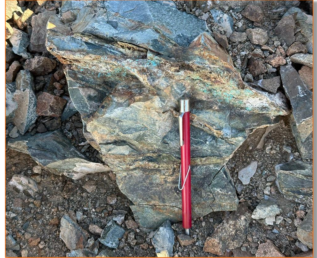
Example of stockwork mineralization exhibiting larger quartz veinlets. The mineralized rock is characterized by multiple veinlets and fractures at various orientations
