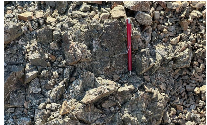
Stockwork with limonites in diorite, with intense argillic-chlorite alteration
