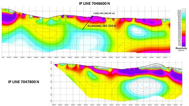
**Figure 4:** IP Survey lines adjacent to the north and south of the Central Zone Target area. Note Hole CAR22-003 is projected onto the section and is collared 200 meters north of the IP line and intersects it obliquely (Figure 2). The large white areas are resistivity highs which would commonly represent most intensely silicified (vuggy quartz) alteration zones, highly prospective for mineralization.
