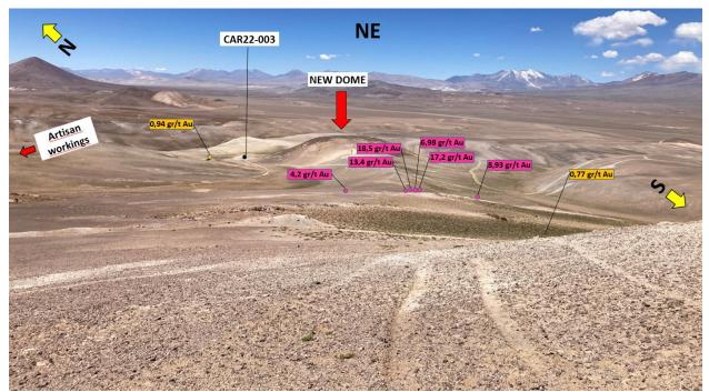
**Figure 3:** Widespread gold mineralization from outcrops and subcrops adjacent to the newly discovered dacitic volcanic dome at the Central Zone Target, Carachapampa Project. The area is pervasively covered by the younger volcanic gravels. However, the limited exposures that protrude through the gravels are commonly mineralized.
