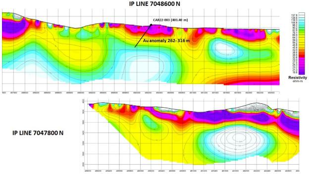
**Figure 4:** IP Survey lines adjacent to the north and south of the Central Zone Target area. Note Hole CAR22-003 is projected onto the section and is collared 200 meters north of the IP line and intersects it
